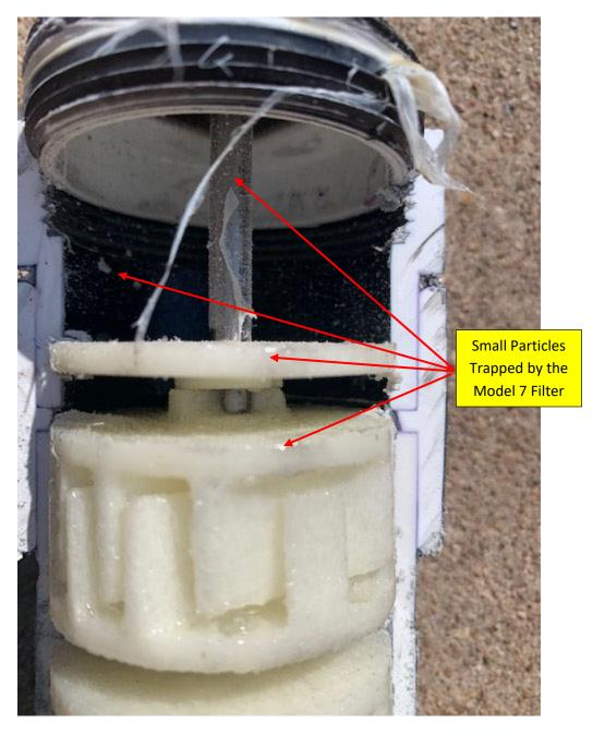
FIGURE 4- MODEL 7 FILTER DISC ASSEMBLY
