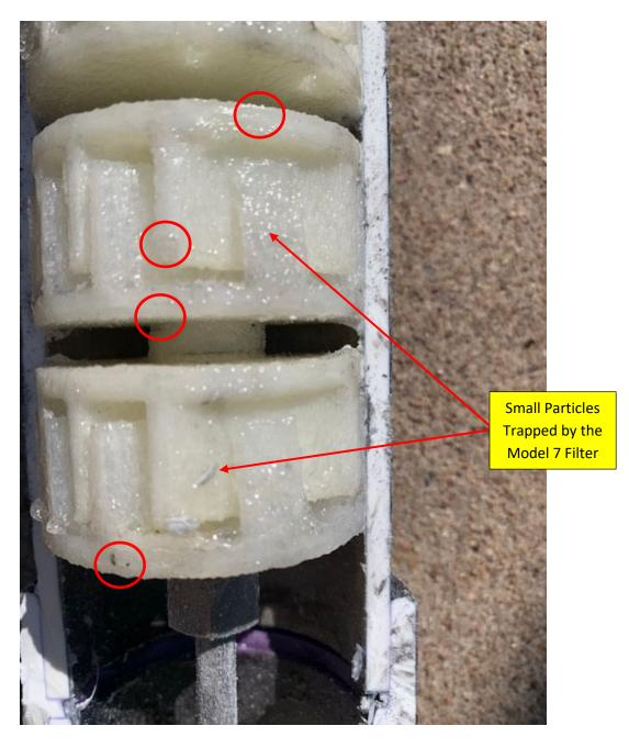
FIGURE 3- MODEL 7 FILTER DISC ASSEMBLY
