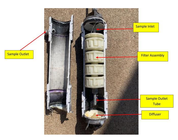
FIGURE 1- MODEL 7 FILTER ASSEMBLY
